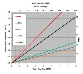
\*All data is based on absolute rated medias. Nominally rated medias will result in a pressure drop reduction of approximately 10%.
