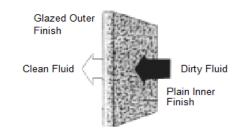
Depth Felt Filter Media Traps Dirt Particles
